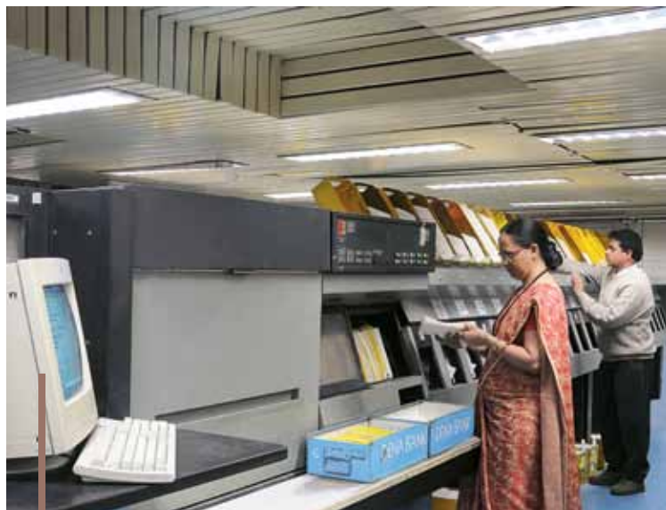
Efficient funds clearing was first initiated in the '80s through Magnetic Ink Character Recognition (MICR) technology.
